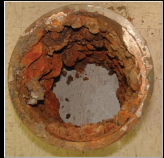
Pipe with buildup of minerals reduces flow through the pipeline. Pigging the pipeline removes this buildup
